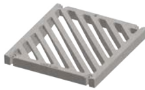
Type M4 Grate Approx. 270 sq. in. open area 2 grates required
